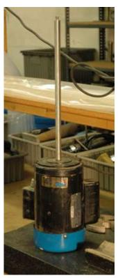
Fig. 1. Position Motor/Shaft Assembly as shown. Secure Assembly, then turn on Motor to determine if Shaft is balanced or unbalanced.
